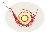
The patented prevents chips from adhering to the screw, ensuring dependable transport of even long shavings.
